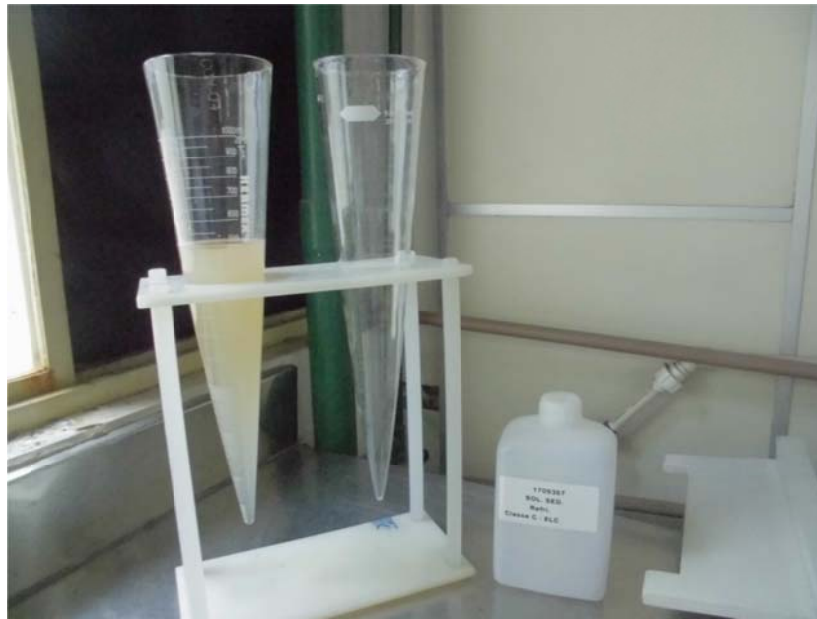
Figure 6 – Imhoff Cone used to determine the amount of sedimentable solids at the CETESB Inorganic Chemistry Lab. Photo: C.L. Midaglia ,2017
