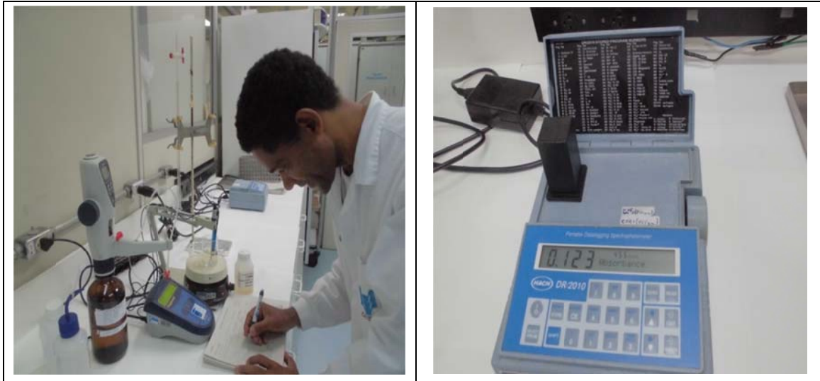
Figure 2 - Procedure for determining color using the spectrophotometer at the CETESB Laboratory of Inorganic Chemistry Photo: R. Rossetti (2017)
