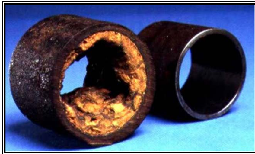
Figure 13- Incrustation of a water pipe (Available at: http://inspecaoequipto.blogspot.com.br/2013/08/inscrustacao-em-caldeiras.html Accessed in August of 2016)
